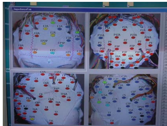
Impedance check of single electrodes in the MEEMM head cap
